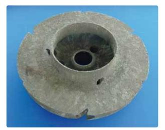
Pump wheel damaged by acid corrosion
