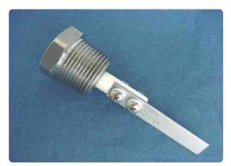
Coupon for corrosion monitoring
