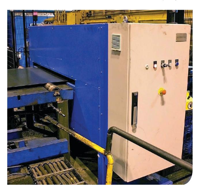
The AWC-1800 is an instrumentation for automatic in-line quality control of welds joining coils for continuous strip processing. The system is designed for non-contact detection of area weight distribution in a strip segment covering the joint weld and the neighbor sector of the joined steel coils. The system can be placed right after the welding machine.
