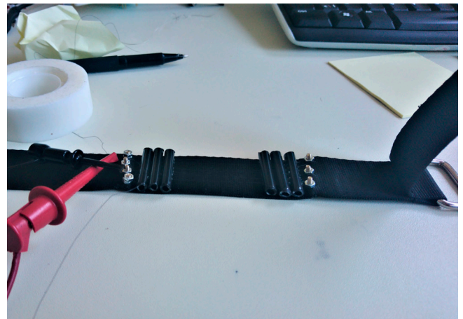
Figure 6: A prototype of the Fibo bracelet with FLEXINOL smartwires.
