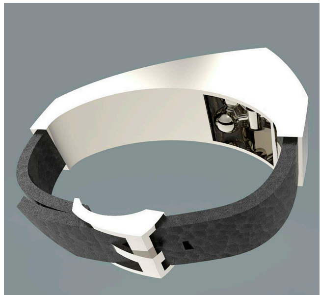
Figure 2: Showing the rotating beads inside the Fibo smart bracelet.
