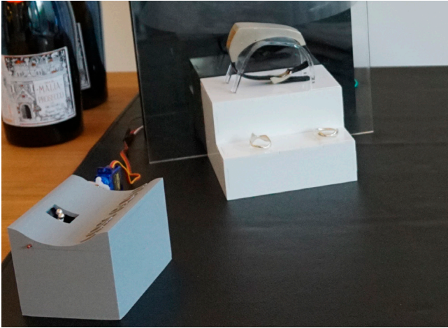
Figure 5: Since a servo motor could not be fitted into the bracelet itself a feel box was created to enable people to feel the beads on their wrist.
