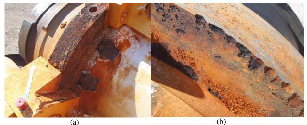
Figure 6: (a) Excessive corrosion on female connector and in spider contact area. (b) Excessive corrosion along edge of female connector.
