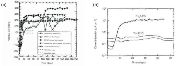
Figure 3: (a) Free corrosion potential of UNS S31254 exposed to seawater [7]. (b) Cathodic current densities vs exposure time for 6 % Mo stainless steel at 7.5 °C and 31 °C at -300 mV SCE[7].
