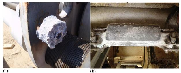
Figure 11: (a) Aluminum anode on guide plate showing 30 % consumption after 340 days exposure. (a) Al-Ga bracelet anode mounted directly on duplex hydraulic line.
