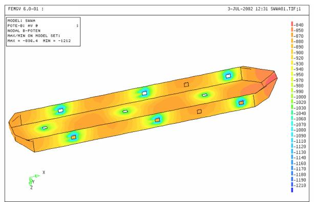
Figure 4 FPSO with 12 ICCP anodes
