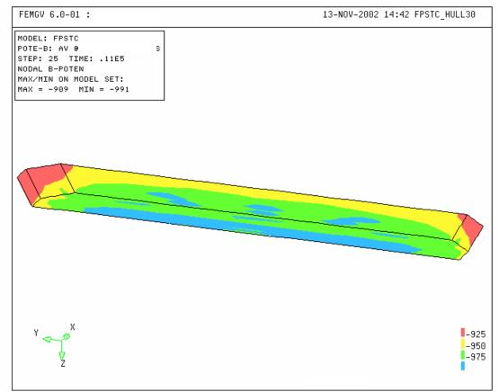
Figure 7 Potential distribution at the end of operational life (30 years) on an FPSO Hull with sacrificial anodes equally distributed on the hull.
