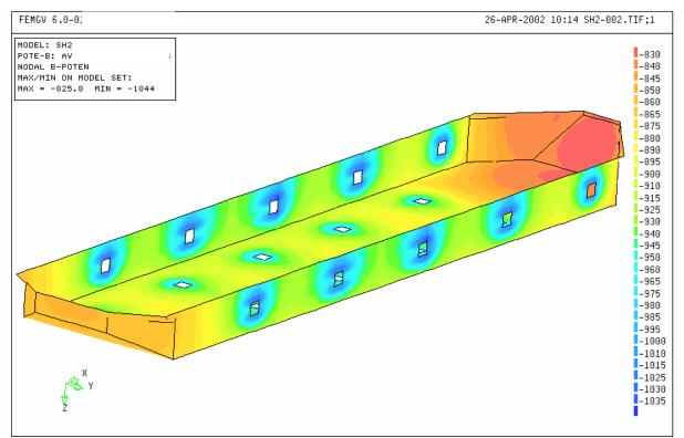
Figure 6 FPSO with 20 ICCP anodes
