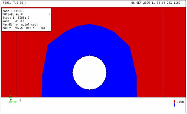
Figure 1 Potential around ICCP anode. The outer of the blue represents -1150 mV. The white circular area represents anode and the initial proposed shield size.
