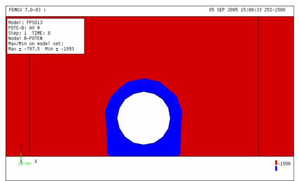
Figure 2 Potential around ICCP anode. The outer of the blue represents -1500 mV. The white circular area represents anode and the initial proposed shield size.
