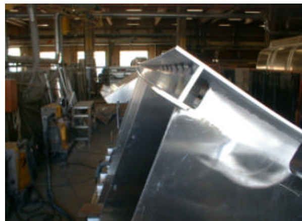
Figur 2.161 Pilhøjde for side-profil, sagging situation.
