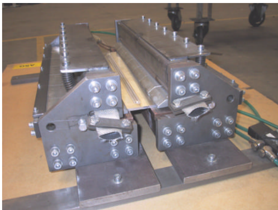
Figur 3.39 Vandkølet specialfikstur (Migatronic).
