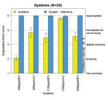
Mean scores with confidence intervals from an ITU-R BS.1116-3 test including 5 systems (degradation compared to reference).
