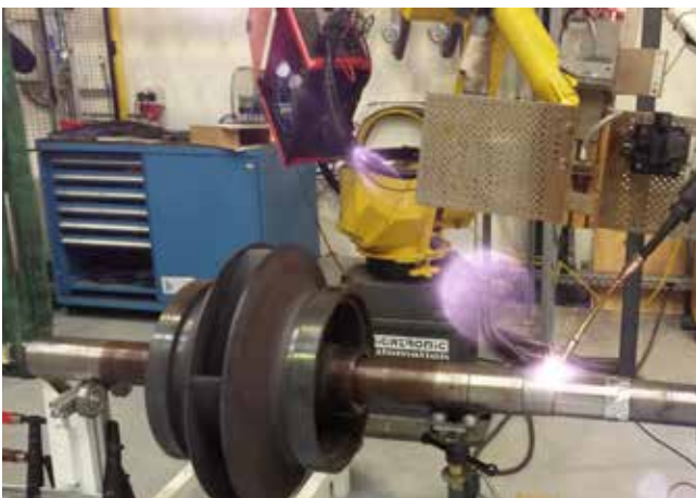
Remanufacturing of pump wheel shaft.
