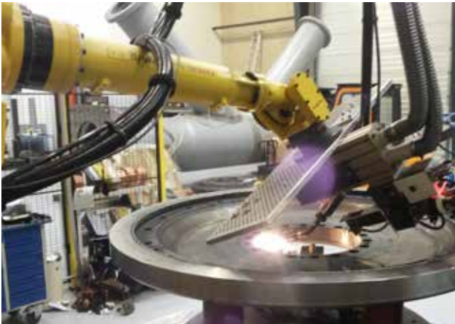
Remanufacturing of ID surface on high value steel component.
