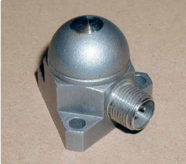
Nd-YAG laser welded accelerometer with pre-mounted sensitive electronics
