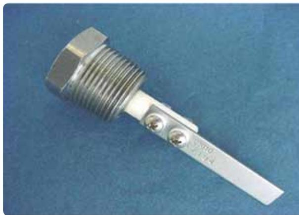
*Coupon for corrosion monitoring*
