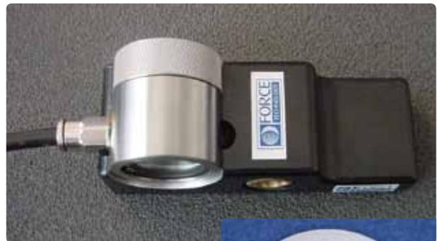
Tint-Tester and test dish for validating shield gas quality for welding
