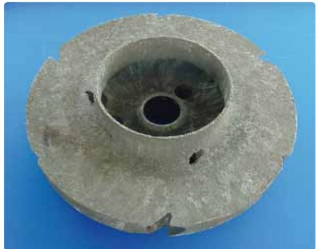
*Pump wheel damaged by acid corrosion*
