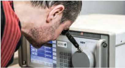
ACCREDITED CALIBRATION OF HUMIDITY SENSORS
