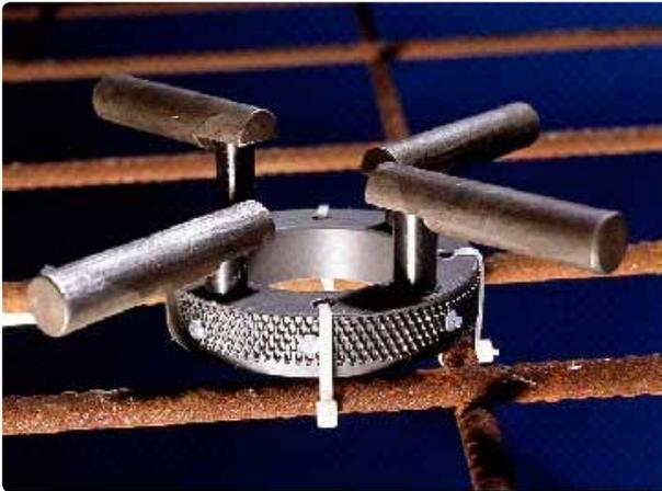
CorroWatch sensor with four anodes
