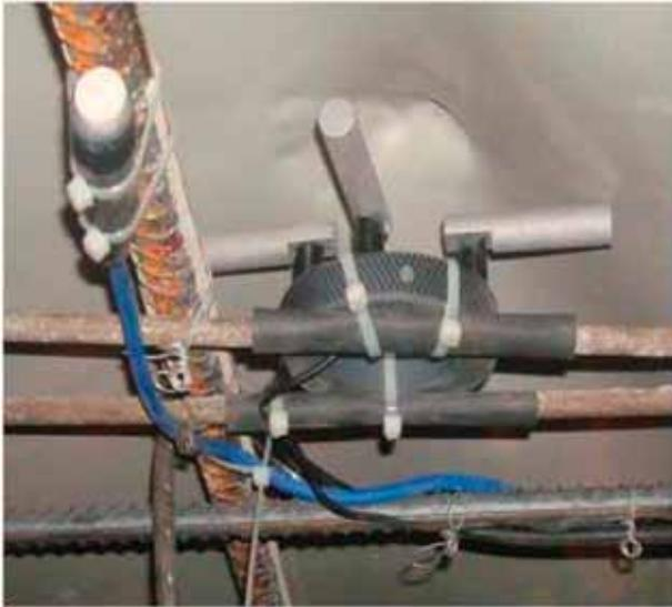
CorroWatch and ERE 20 prepared for measurements with Camur II system
