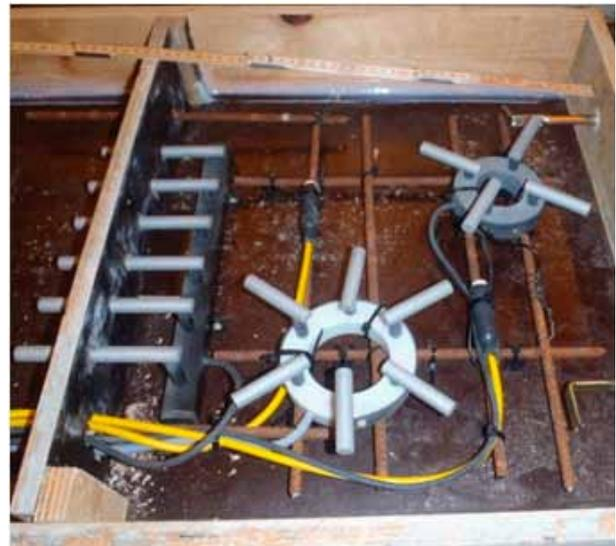
CorroWatch with six and four anodes and staircase sensor for casting joint measurements
