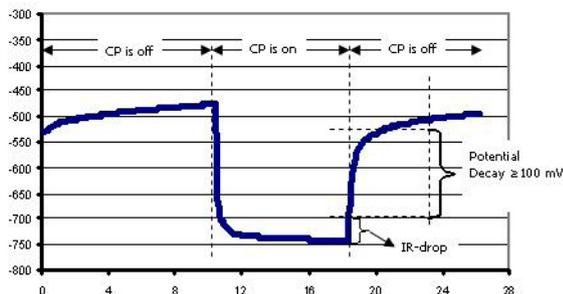
Check of cathodic protection by means of potential decay criterium
