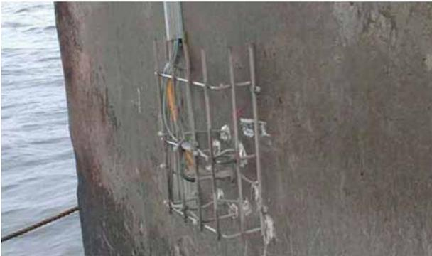
Photo of CorroRisk installation on marine bridge pillar
