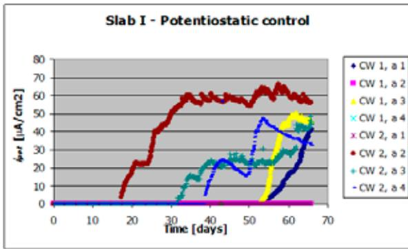
CorroWatch measurements of corrosion current
