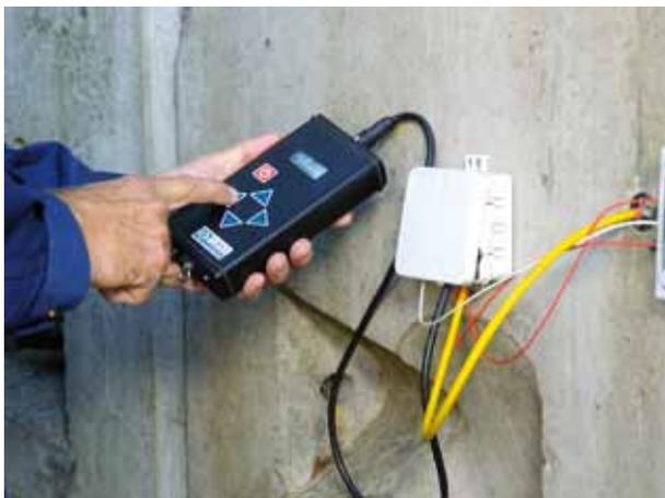
CorroZoa under measurements on site
