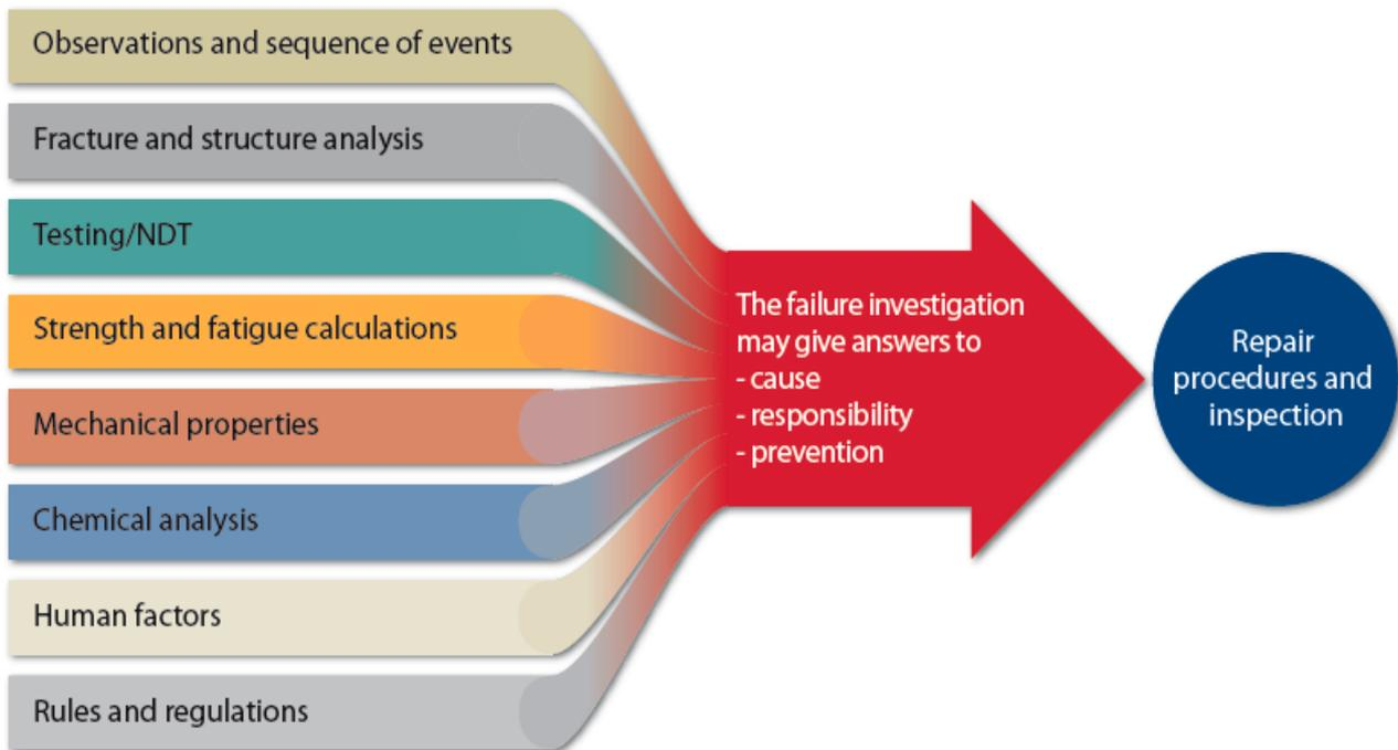
A failure and damage investigation may be dealt with in many ways, depending on the requirements to be met. Sometimes it requires only few and simple examinations to clarify specific technical questions and sometimes a more thorough examination is required, to determine causes etc., called Root Cause Analysis (RCA).
