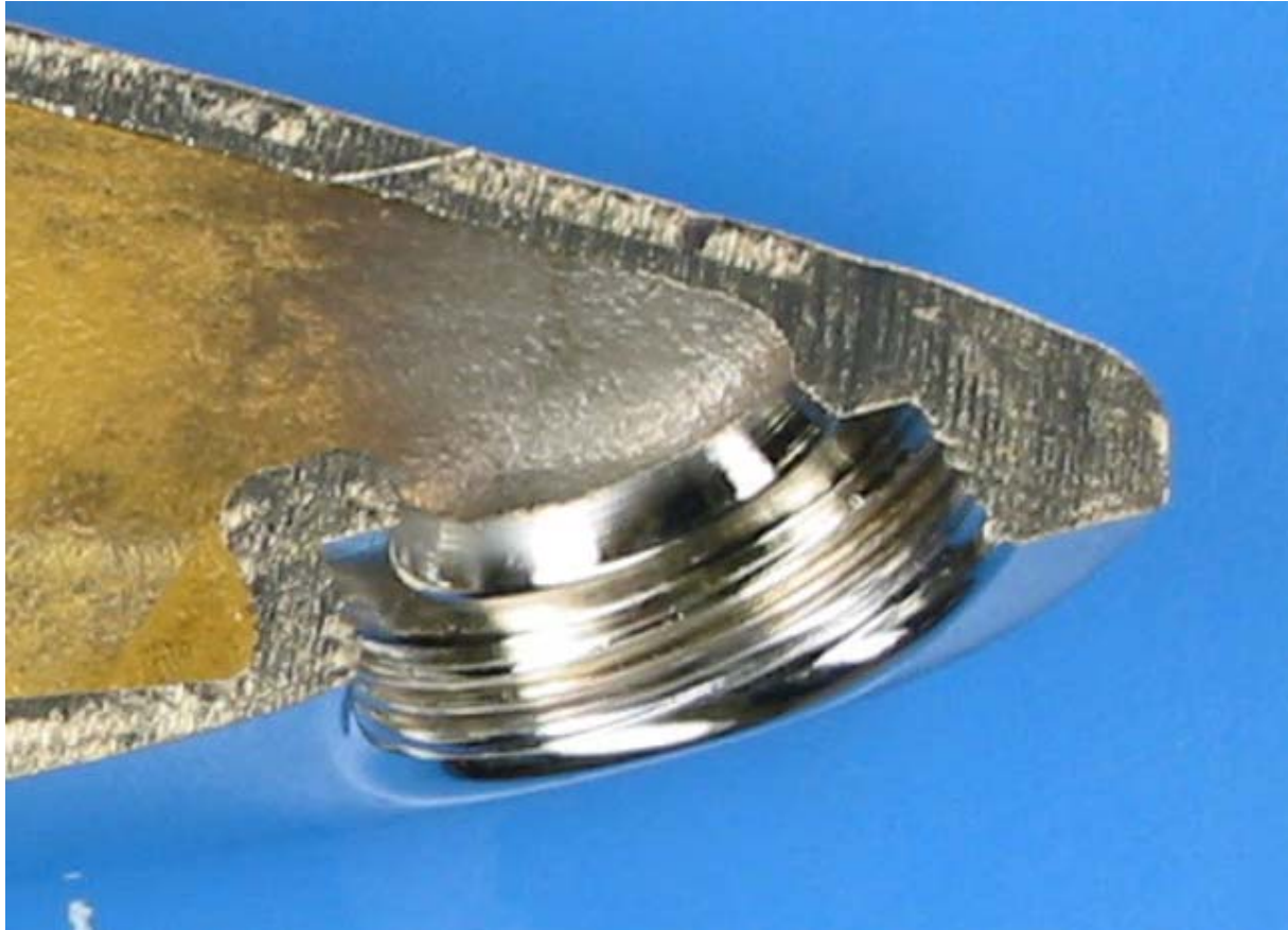
Figure 2: Close-up of aperture on mixer tap spout showing nickel at the inside.
