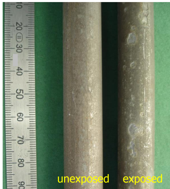
FIGURE 10: Cleaned surface of full-length coupon showing only minor corrosion after 1 year' exposure.
