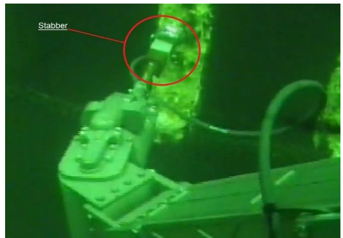
FIGURE 12: Potential measurement using a stabber (contact reference cell) mounted on a ROV.
