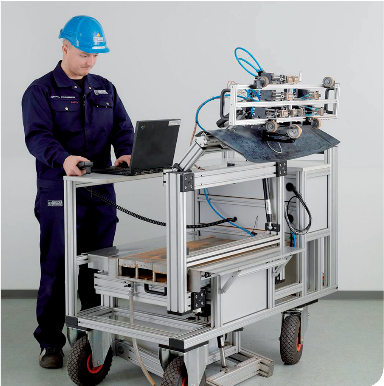
AMS-41 set-up for scanning of butt weld
