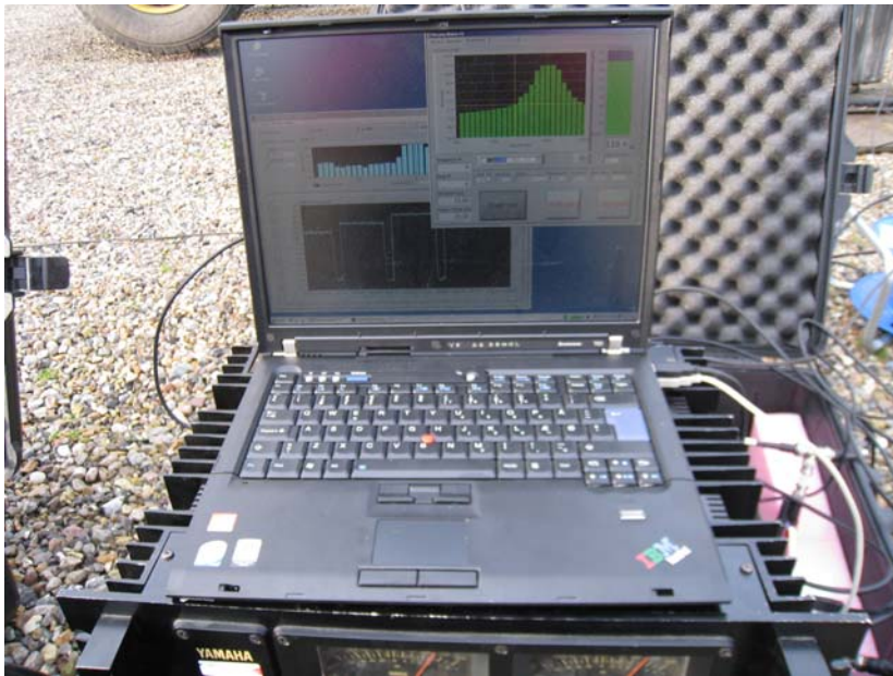
Figure 3 The noise generator and the noiseLAB recorder were running on the same laptop. The noise generator is top left on the computer display and the recorder bottom left. The “stripchart” on the recorder shows the sequence with noise on and noise off. The amplifier is seen under the laptop.
