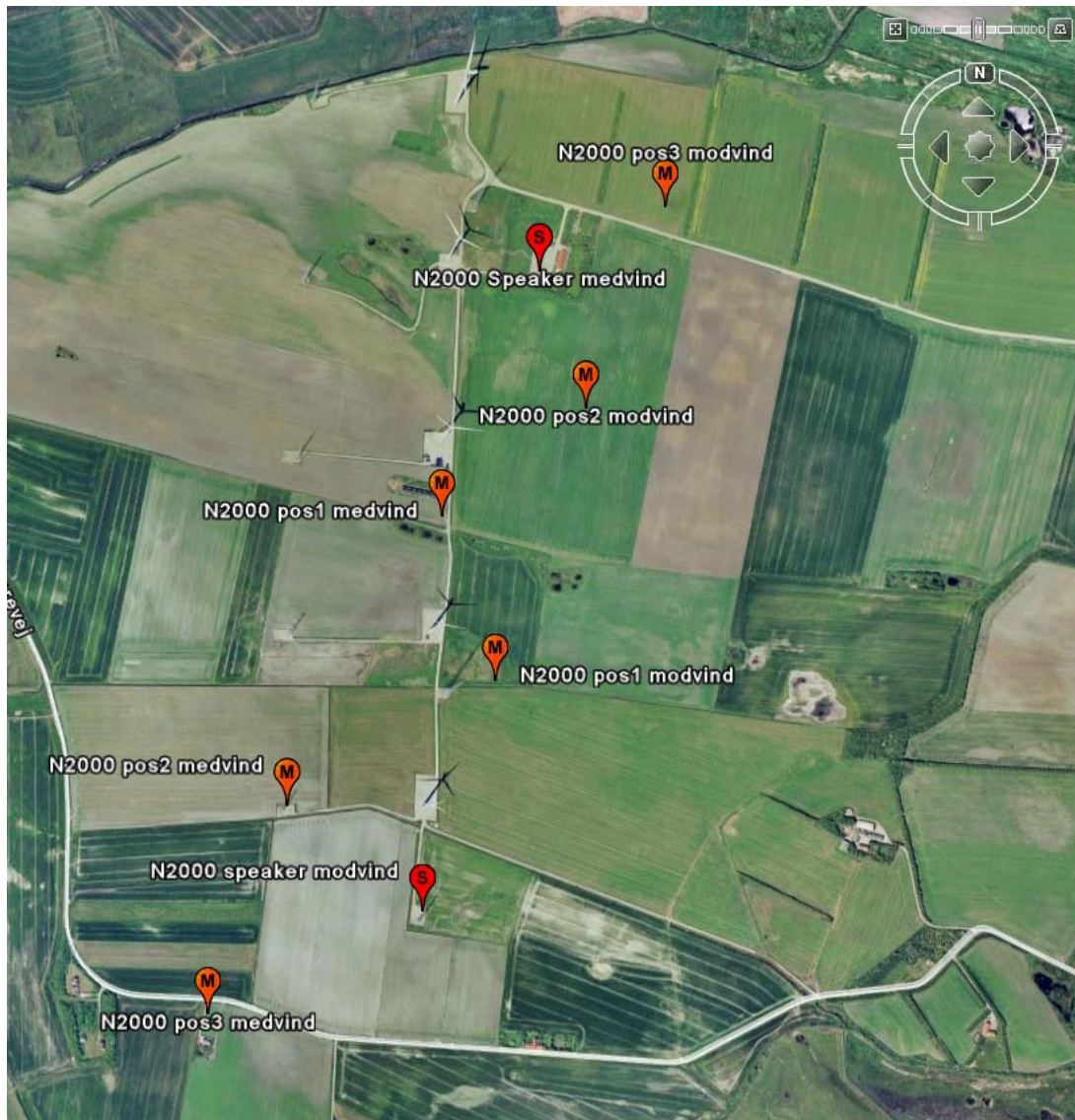
Figure 2 Høvsøre test site. The loudspeaker position was changed between downwind and upwind measurements. The terrain is flat and typically agricultural. The indicators marked S are source positions and M are receivers. “medvind” means downwind and “modvind” is upwind.
