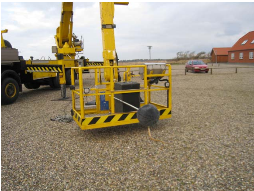
Figure 4 Mounting of the loudspeaker and the microphone in front of the loudspeaker for the Høvsøre measurements. The elevation of the loudspeaker was 50 m and 30 m during measurements.
