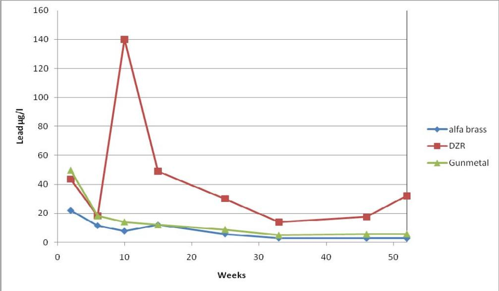
Fig. 3. Lead release after 12 hours stagnation from machined test pieces of alfa brass, dezincification resistant brass (DZR) and gun metal. Average of two data sets.
