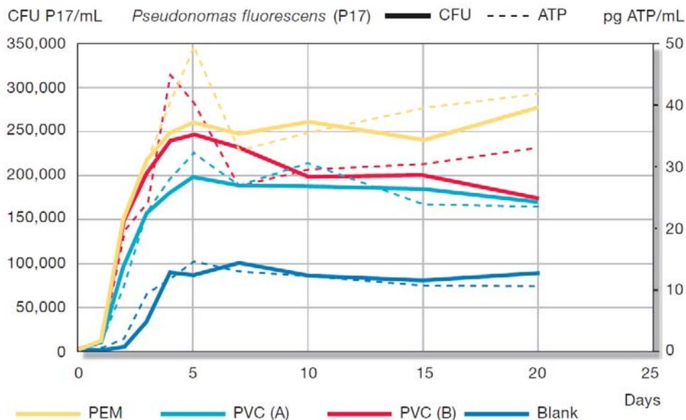
Fig. 7. Growth measured by HPC and ATP of the bacteria strain P17 at 15 °C in drinking water extracts of two types of PVC, a PEM material, and in blank (water alone).[7]
