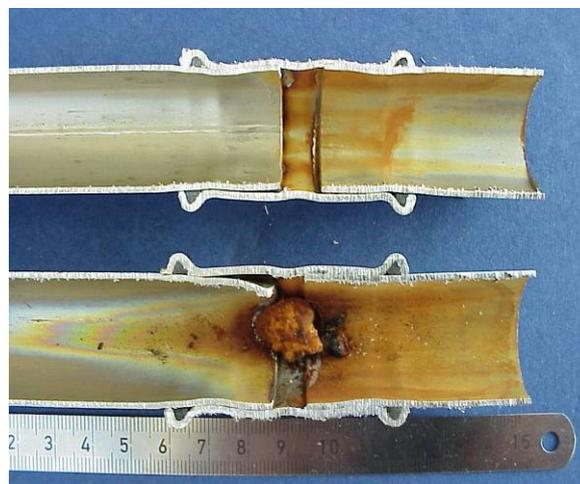
*Fig. 4. MIC in press fitting, stainless steel 1.4401 after approximately 1 year exposure.*
