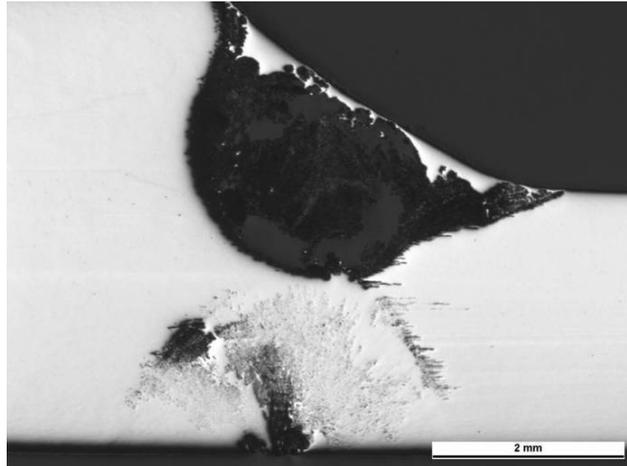
Fig. 6. Cross section through the corrosion attack in Fig. 5. Internal weld pass is fully dissolved by corrosion, the external weld being porous from selective attack in the ferrite phase.
