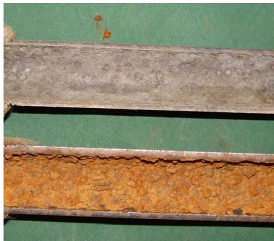
*Fig. 2 Hot dip galvanised steel pipes from warm water installations, 40-50 years old. On top half scale has been cleaned off.*
