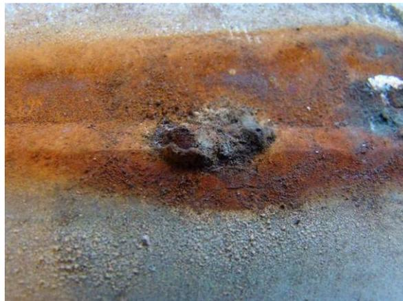
*Fig. 5. Corrosion attack with corrosion products as blister and thin layers of rust spreading from it - starting at the weld. Water side of heating jacket.*
