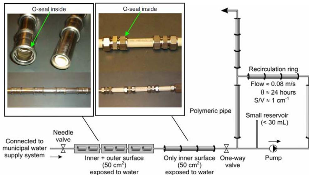
*Fig. 8. Continuous flow model system for investigating biofilm formation on polymers [13,14].*
