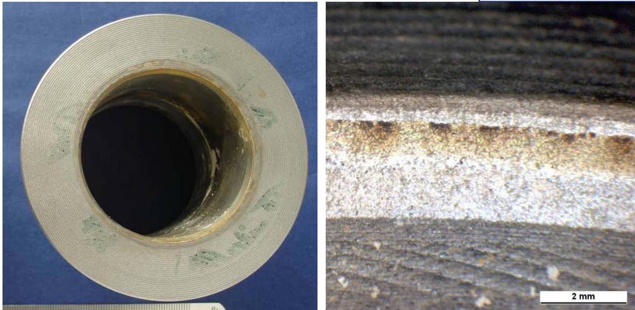
**Figure 8:** Overview of flange face from the FRG gasket test (left). Close-up of superficial corrosion on flange face (right).
