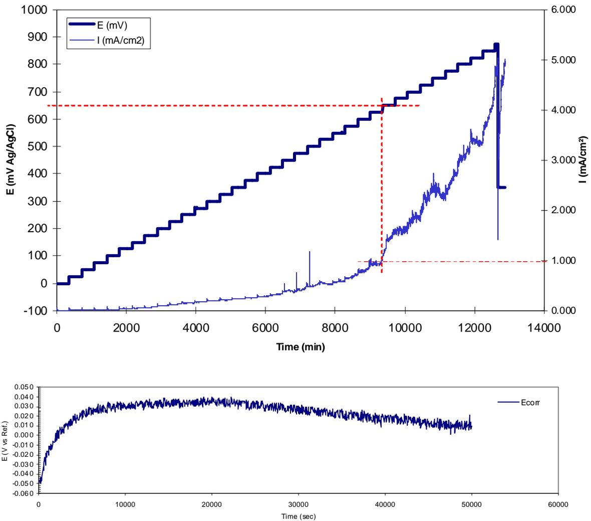
**Figure 3:** Current and potential measurements of graphite gasket. Corrosion initiates at +750 mV Ag/AgCl. Curve at the bottom represents potential measurement prior to polarisation.
