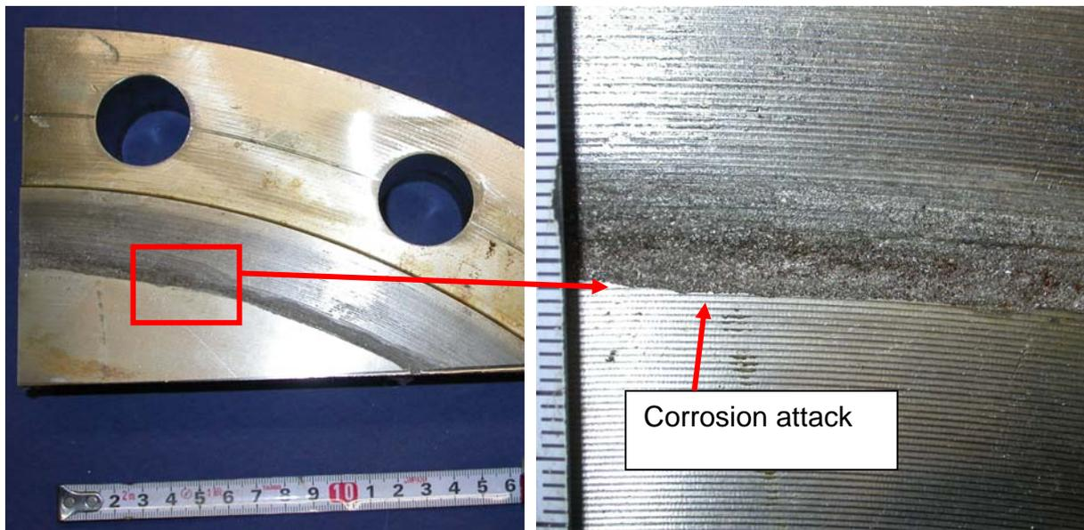
**Figure 1:** Failure investigation of crevice corrosion in 6Mo flange after 1 years of service in a firewater system.
