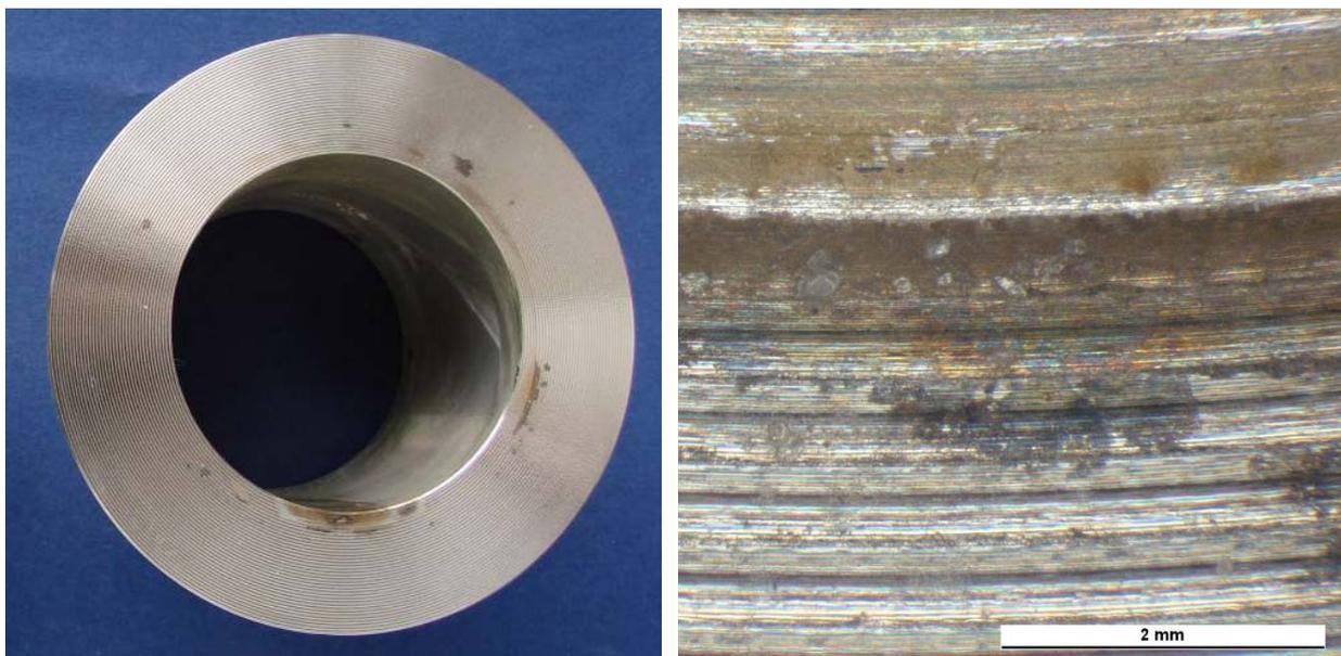
**Figure 9:** Overview of flange face from the Klingersil C4430 gasket test (left). Close up of superficial corrosion on flange face (right).
