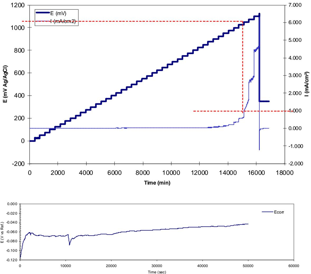
**Figure 4:** Current and potential measurements of FRG gasket. Corrosion initiates at +1050 mV Ag/AgCl. Curve at the bottom represents potential measurement prior to polarisation.
