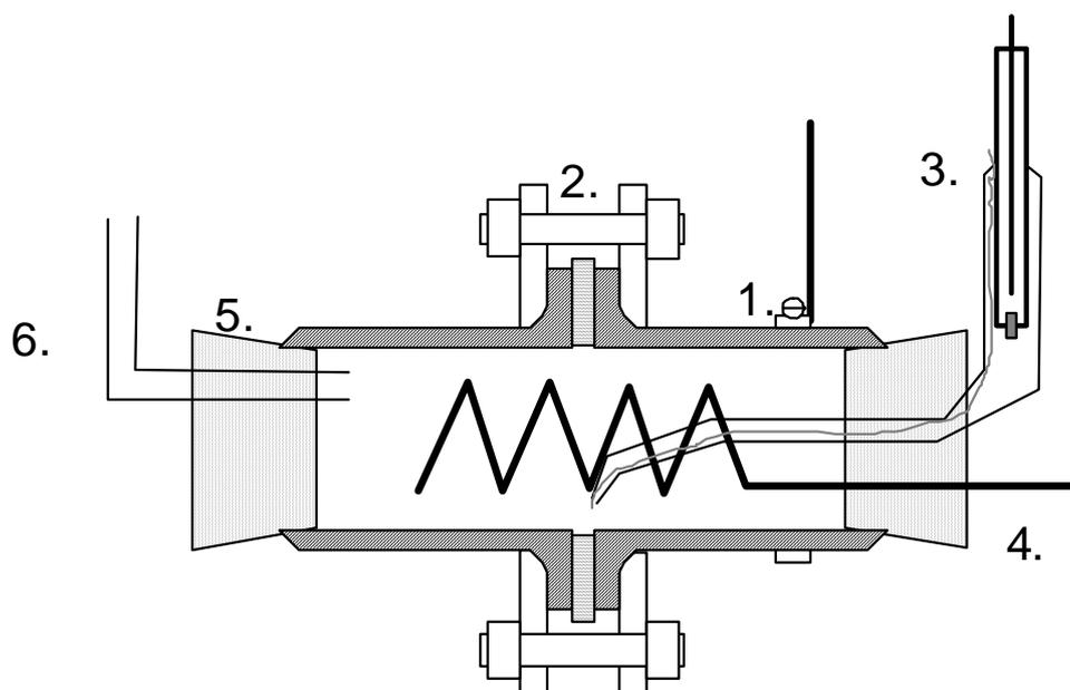
**Figure 2:** Test set-up: 1. Stub end 2", 6Mo, electrical contact at hose clamp. 2. Flange and gasket. 3. Reference electrode (Ag/AgCl/sat.KCl) in salt bridge with cord to avoid air bubbles. 4. Hastelloy C276 counter electrode. 5. Silicone rubber stopper. Zinc oxide paste is applied at contact face to prevent crevice corrosion. 6. Filling tube.
