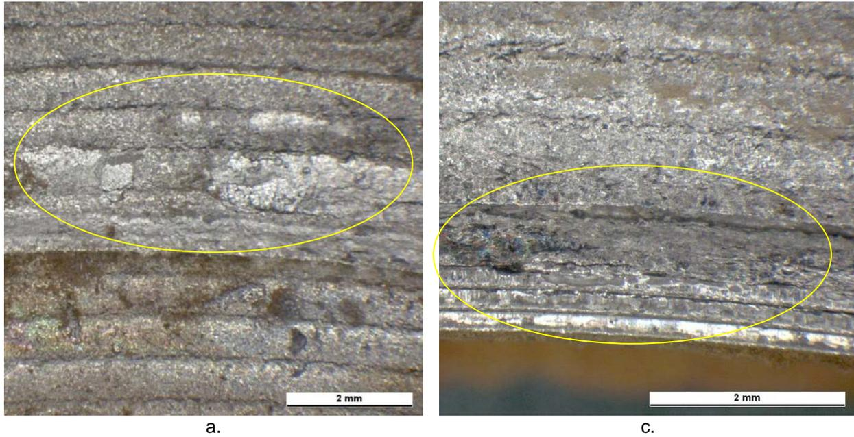
**Figure 6:** Close-up of superficial corrosion in outer grooves on 6Mo flange face (a) and deeper corrosion along edge in outer windings of duplex spiral in the graphite gasket (b).
