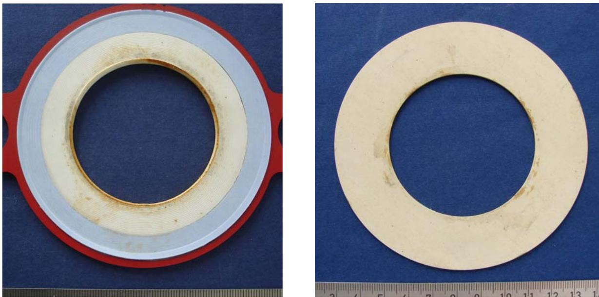
**Figure 7:** Overview of FRG gasket (left) and Klingersil C4430 gasket (right) after test.
