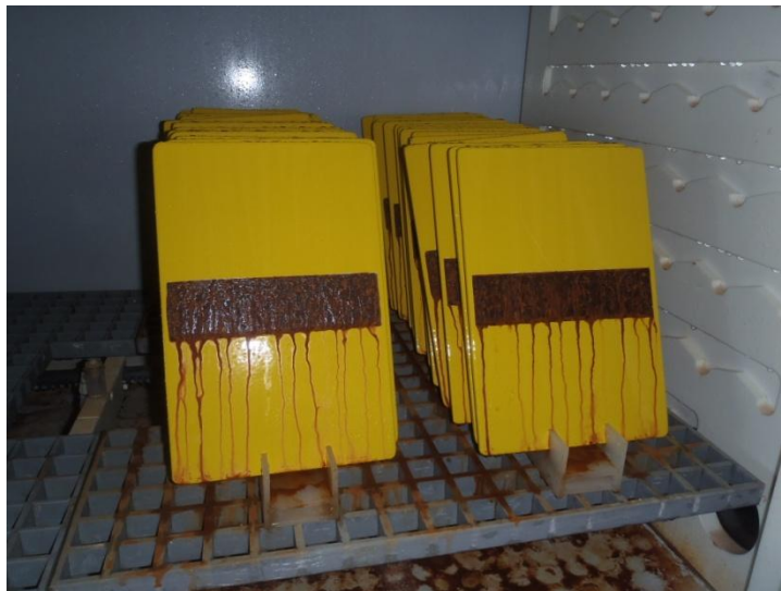
Figure 1: Panels in neutral salt spray chamber during pre-rusting.
