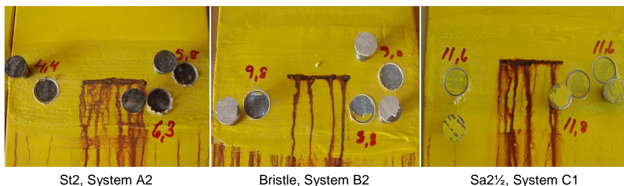
Figure 5: Examples of adhesion test results including dollies after neutral salt spray test.
