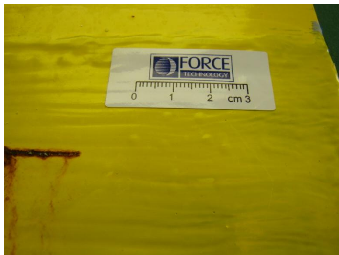
Figure 3: Example of blistering after neutral salt spray test. Result: 3(S4) (St2, System C2).
