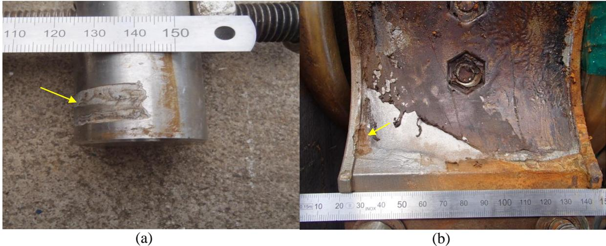
Figure 9: (a) Crevice corrosion below strap on UNS S31603 tensioner for buoyancy module. (b) Crevice corrosion inside a clamp of UNS S31603.
