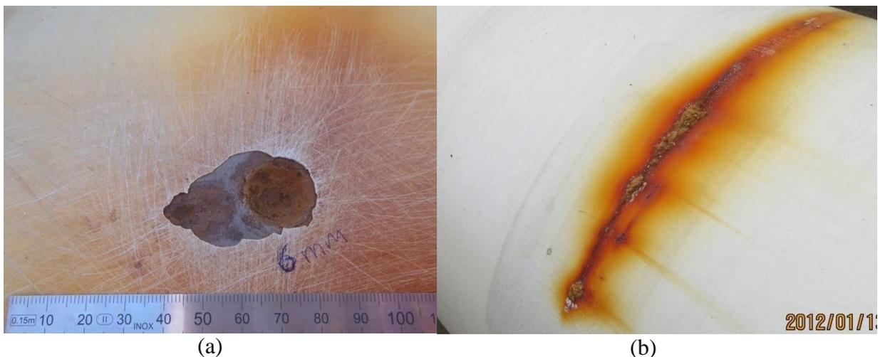
Figure 8: (a) Severe pin-hole corrosion on main pipe due to paint defect. The measured depth is 6 mm. (b) Line of coating defects on main pipe from contact with buoyancy module.
