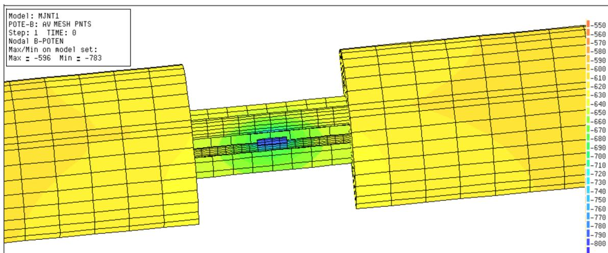
Figure 12: Example of CP modeling to calculate the required number of anodes for depolarizing the stainless steel line.
