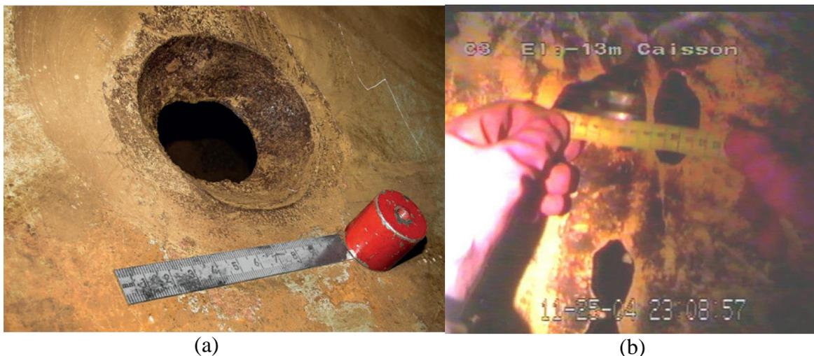
Figure 4: Examples of severe galvanic corrosion of paint coated steel due to influence from corrosion resistance alloy; (a) stern tube in ship (b) seawater pump caisson [9].
