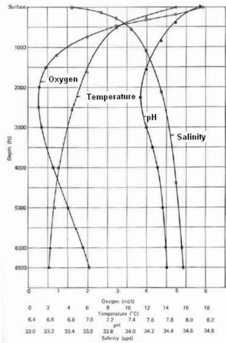
Figure 2: Variations in seawater with depth at a Pacific Ocean test site [2].
