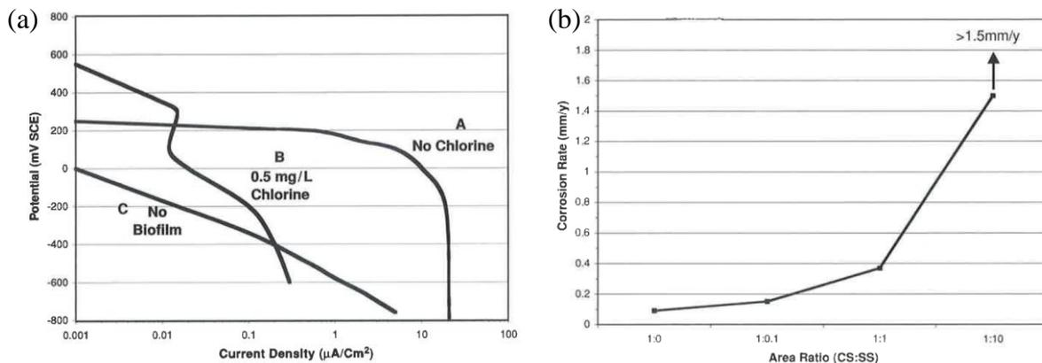
Figure 5: (a) Cathodic polarization curves for high-alloy stainless steel in three types of seawater [8]. (b) Corrosion of carbon steel coupled to 6% Mo stainless steel vs. area ratio in natural seawater [8].
