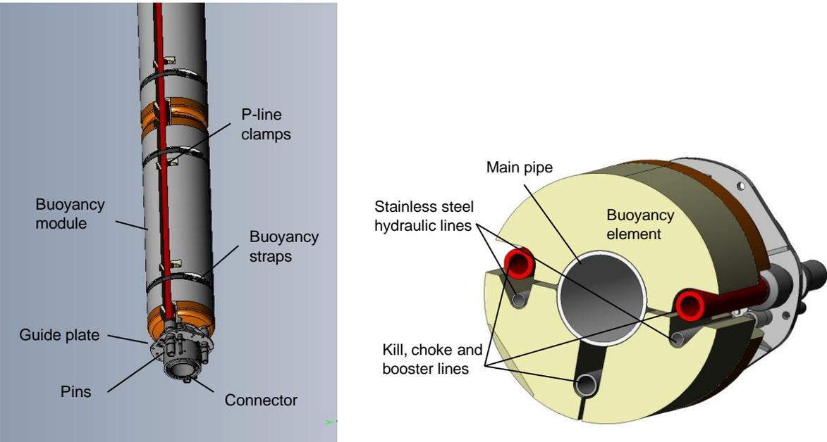
Figure 1. Example of typical marine riser design.
