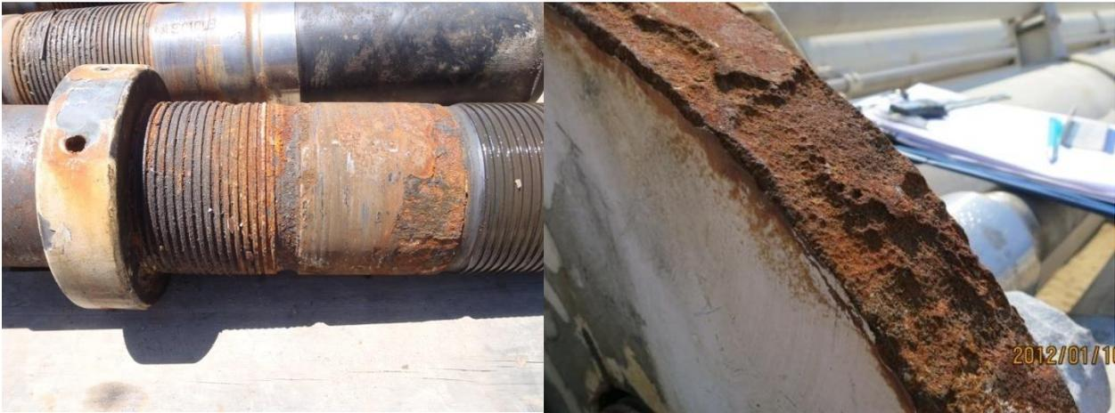
Figure 6: (a) Corrosion on pin for Choke & Kill line. (b) Excessive corrosion along edge of guide plate.
