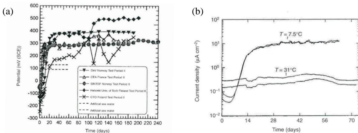
Figure 3: (a) Free corrosion potential of UNS S31254 exposed to seawater [7]. (b) Cathodic current densities vs exposure time for 6 % Mo stainless steel at  $7.5\text{ }^{\circ}\text{C}$  and  $31\text{ }^{\circ}\text{C}$  at  $-300\text{ mV SCE}$ [7].
