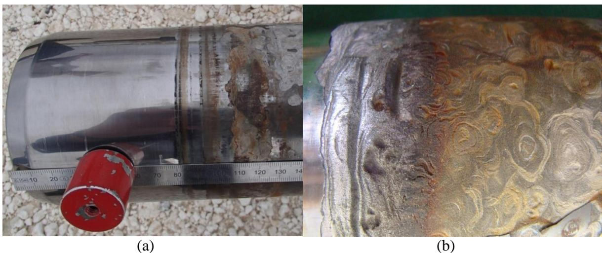
Figure 10: (a) Corrosion of freely exposed Co-Cr-WC hardfacing on pin. (b) Close-up of damage.
