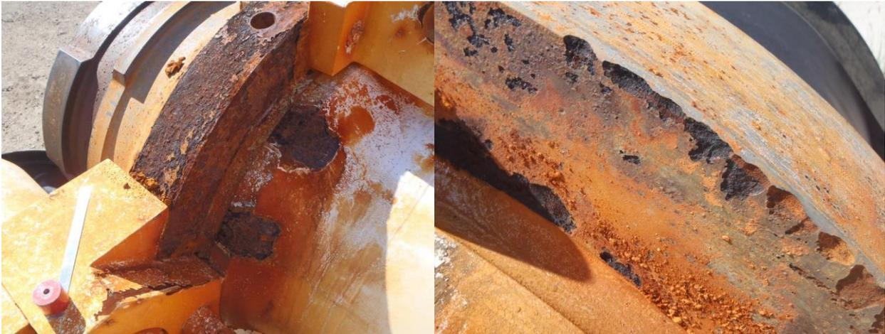
Figure 6: (a) Excessive corrosion on female connector and in spider contact area. (b) Excessive corrosion along edge of female connector.
