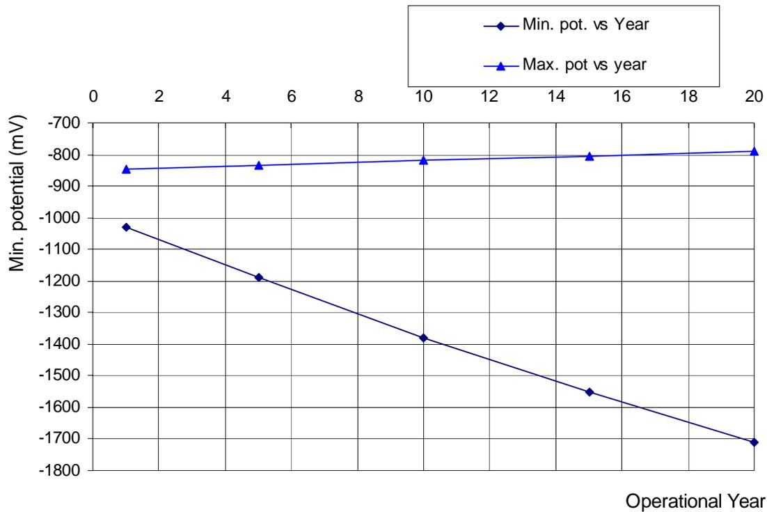
**Figure 8 Development of maximum and minimum potential on an FPSO over 20 years. Minimum potential is on the border of the shielding.**
