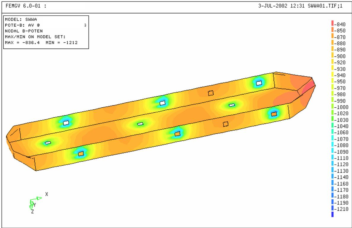
**Figure 4 FPSO with 12 ICCP anodes**
