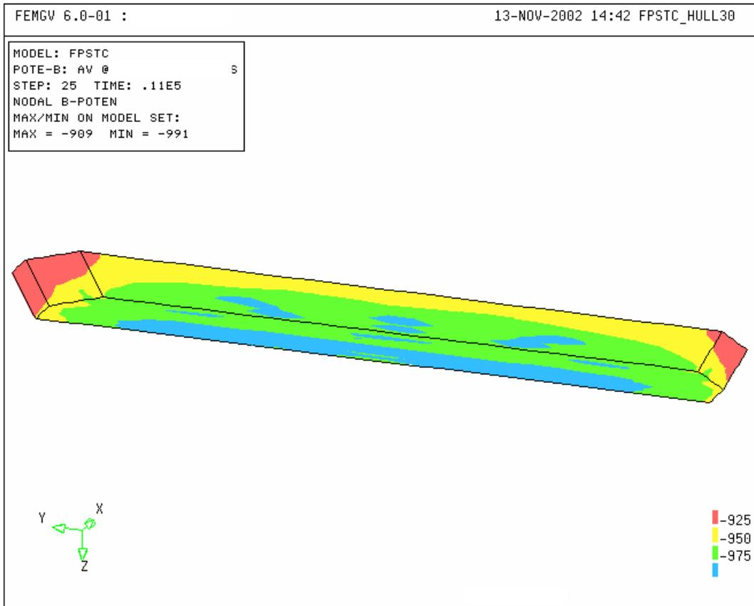
**Figure 7 Potential distribution at the end of operational life (30 years) on an FPSO Hull with sacrificial anodes equally distributed on the hull.**
