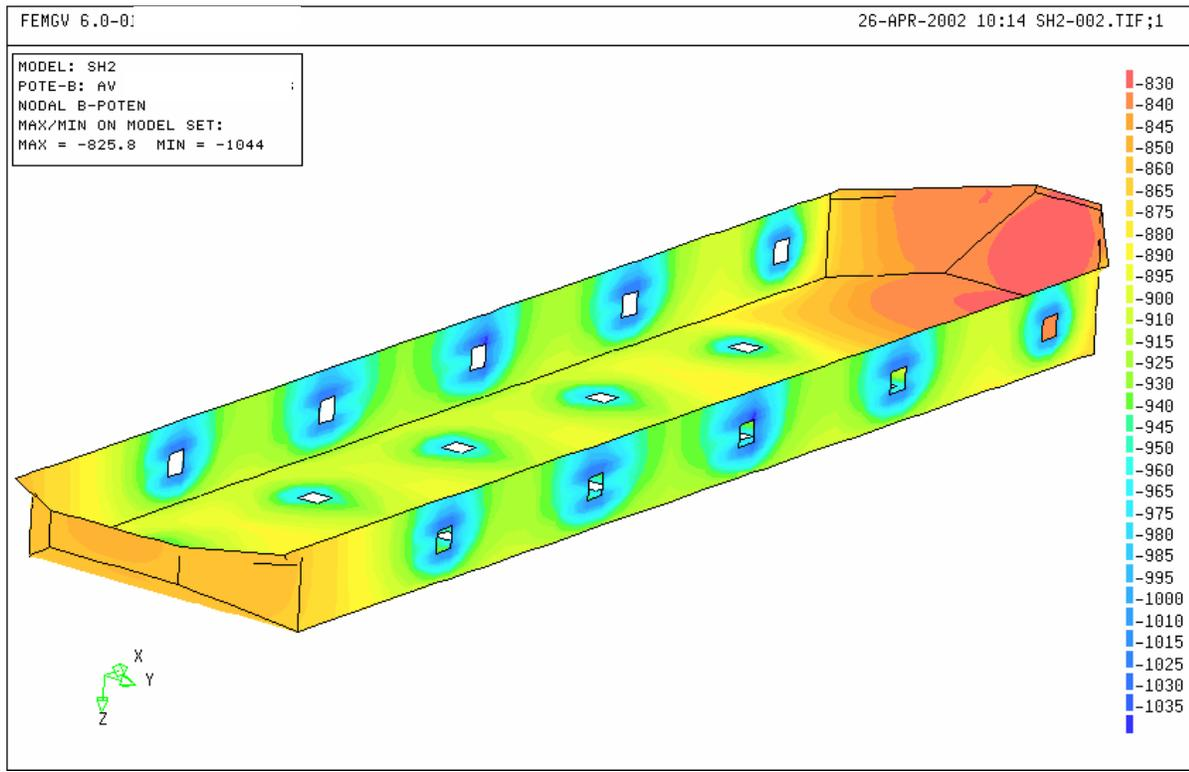
Figure 6 FPSO with 20 ICCP anodes
