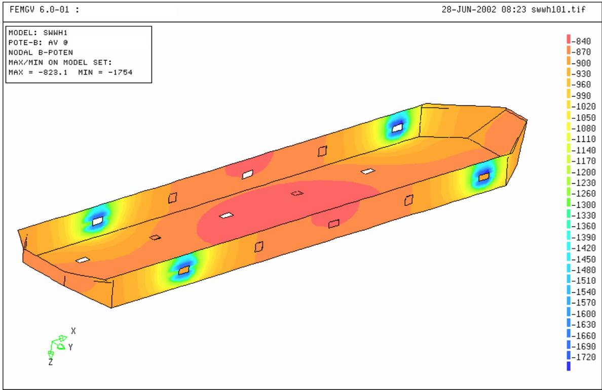
**Figure 3 FPSO with 4 ICCP anodes**
