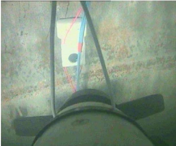
**FIGURE 14:** Magnet mounted zinc reference electrode seen from the actuator used for installing the probe inside the monopile.
