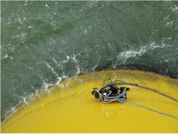
**FIGURE 7:** Thickness measurement by UT-crawler on the external side of transition piece by remotely controlled equipment.
