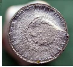
High-strength bolt suffering hydrogen induced cracking (HISC)
