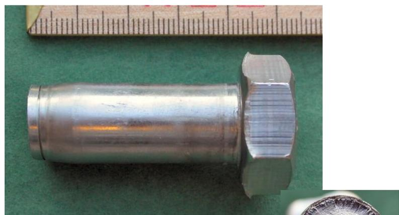
Stainless bolt suffering corrosion fatigue due to poor tightening
