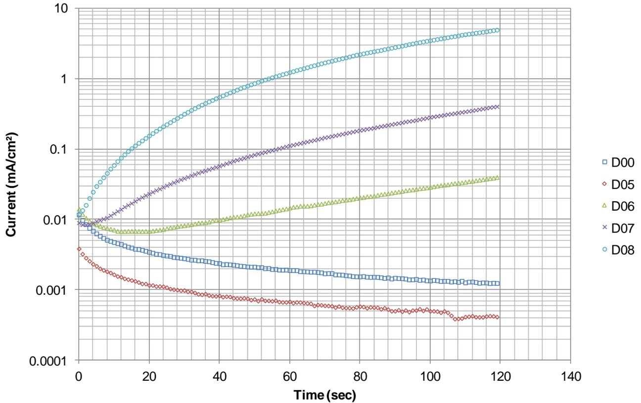
Figure 7: Development in corrosion current at 700 mV SCE and 25 °C when testing UNS S31803 stainless steel heat-treated at 850 °C for 10 and 60 minutes.
