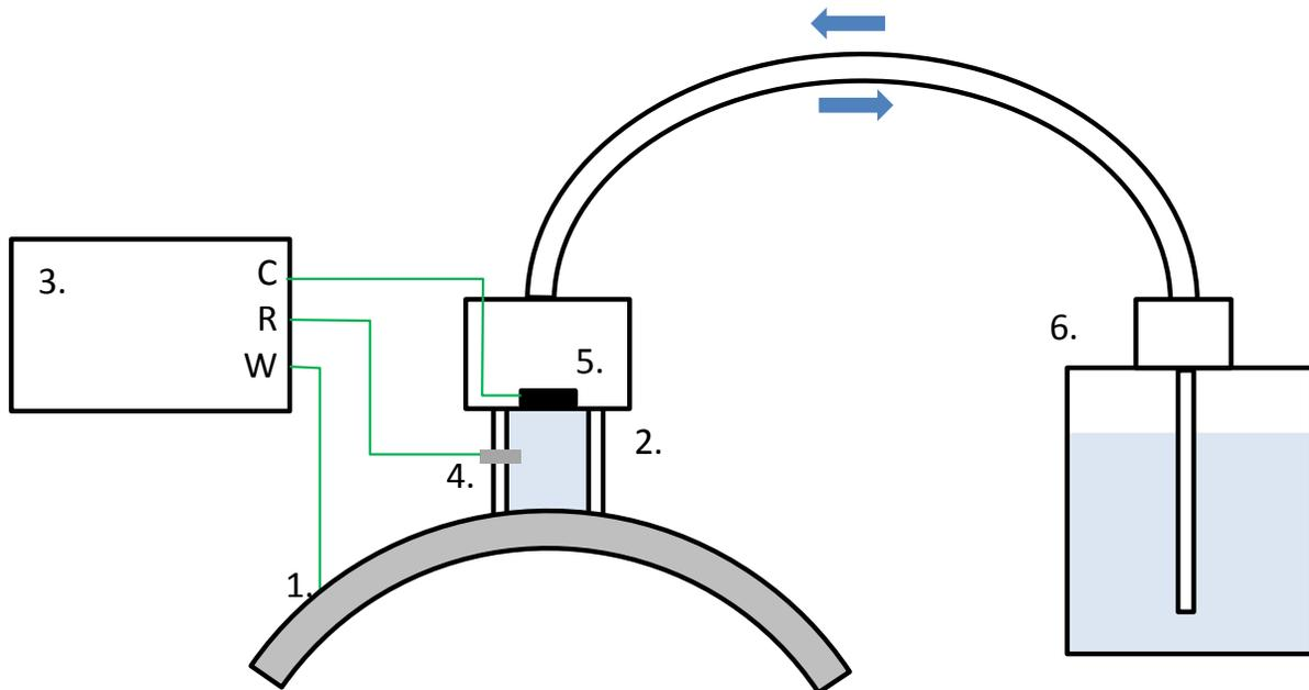
Figure 1: Set-up used for rapid testing. 1. specimen 2. cell (ID 10 mm) made from flexible rubber hose 3. potentiostat 4. silver/silver chloride reference electrode 5. counter electrode 6. pump.
