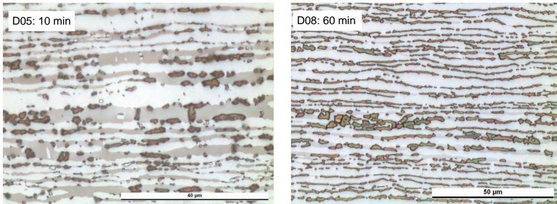
Figure 3: Microstructure of UNS S31803 stainless steel heat-treated at 850 °C for 10 and 60 minutes. Electrolytically etched with NaOH.
