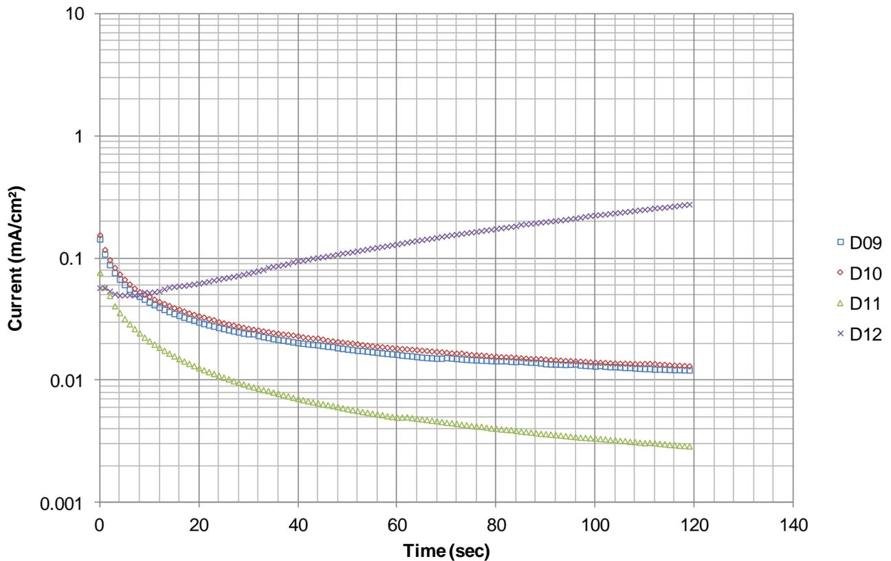
Figure 8: Development in corrosion current at 700 mV SCE at 25 °C when testing duplex stainless steels. D12 contains sigma phase while the other materials are considered healthy.
