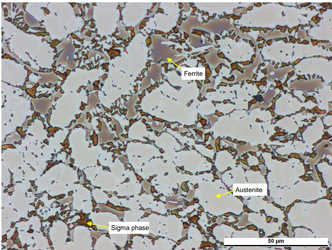
Figure 4: Microstructure of UNS S32750 steel (D12) showing excessive sigma phase precipitation. Electrolytically etched with NaOH.
