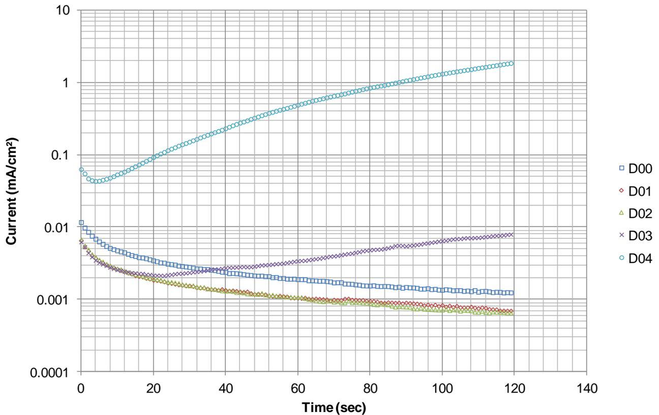
Figure 6: Development in corrosion current at 700 mV SCE and 25 °C when testing UNS S31803 stainless steel heat-treated at 750 °C for 10 and 60 minutes.
