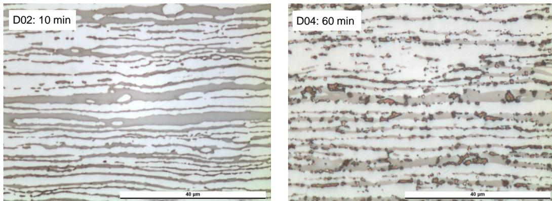
Figure 2: Microstructure of UNS S31803 stainless steel heat-treated at 750 °C for 10 and 60 minutes. Electrolytically etched with NaOH.
