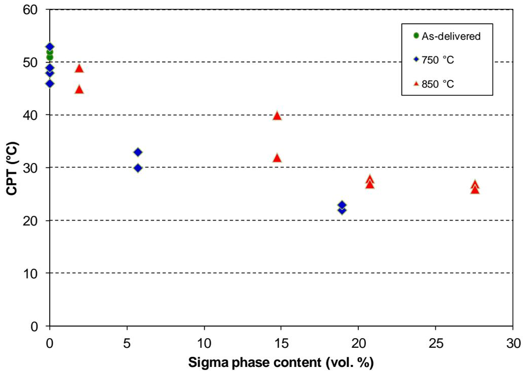
Figure 5: Influence of sigma phase content on CPT of UNS S31803 heat-treated at 750 and 850 °C.
