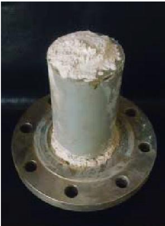
FIGURE 10 - Anode SW08 after removal. Deposits building up on the anode top surface may explain the declining potential drop readings.
