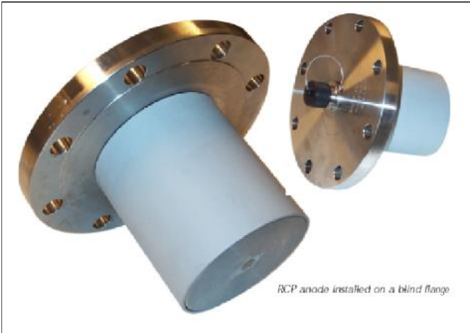
FIGURE 5 - RCP anodes fixed to a blind flange. Only the anode front surface is exposed to the seawater. Connector for potential drop readings is behind the black cap.
