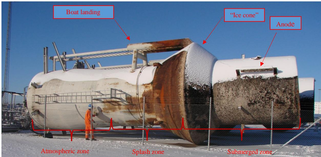
**Figure 6. A decommissioned monopile (2016) from Yttre Stengrund in the Baltic Sea.**
