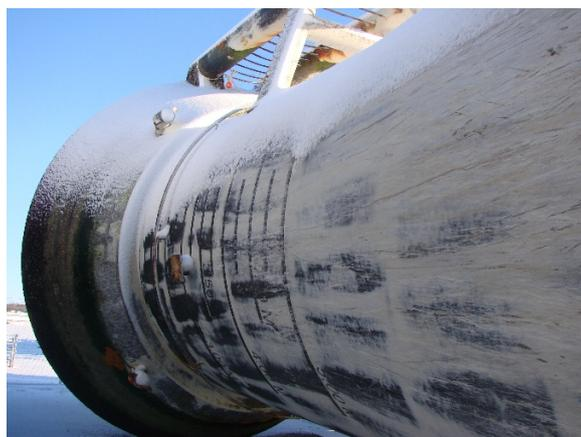
**Figure 7. Erosion pattern of the top layer of the coating system in the splash zone.**
