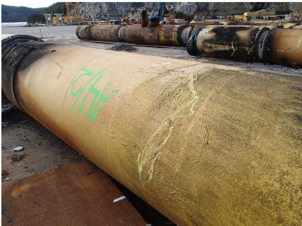
**Figure 8. Inspection of jacket legs from a 40-year old platform at a decommissioning yard. Good adhesion of splash zone coating is observed by scribing with a slag hammer.**
