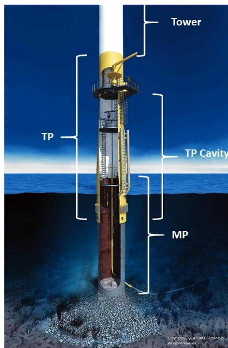
**Figure 1: Offshore wind turbine construction, model: Tower, TP (Transition Piece), TP Cavity (The inner void of the TP), and MP (Monopile: The underwater support of the TP and Tower).**
