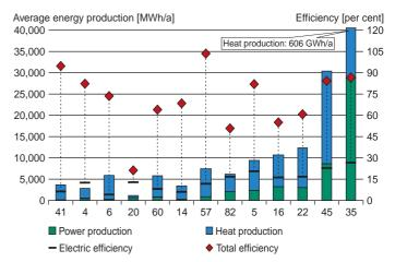
Operational efficiencies for 13 grate fired biomass CHP systems compared to the size of the plant shown as the annual production of electricity and heat. Operational figures are average values for 24 months, September 2003 to August 2005.
