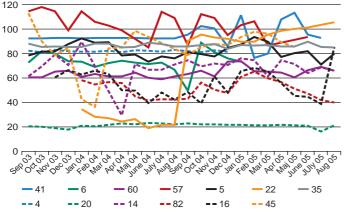
Total of heat and electric efficiencies for 13 grate fired biomass CHP systems. Operational figures are monthly data shown for 24 months, September 2003 to August 2005
