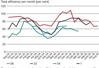
Total of heat and electric efficiencies for 4 biomass gasifier CHP systems. Operational figures are monthly data shown for 24 months, September 2003 to August 2005.
