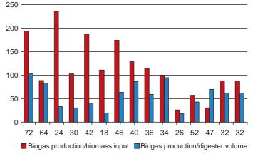
Biogas production relative to the volume of biomass input and to the digester capacity for 15 biogas CHP systems (landfill gas systems not shown here). Operational figures are monthly data shown for 24 months, September 2003 to August 2005.
