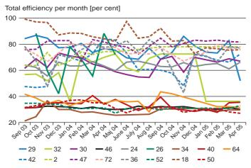
Total of heat and electric efficiencies for 19 biogas and landfill gas CHP systems. Operational figures are monthly data shown for 24 months, September 2003 to August 2005.
