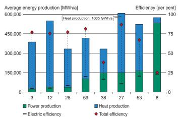
Operational efficiencies for 8 grate fired biomass CHP systems compared to the size of the plant shown as the annual production of electricity and heat. Operational figures are average values for 24 months, September 2003 to August 2005.
