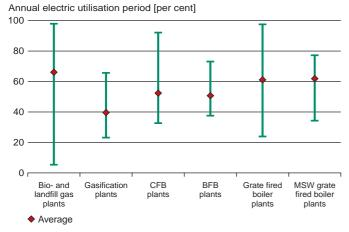
Comparison of the utilisation factor for the different technologies, based on operational data for 24 months Gasification plants perform significantly poorer than the other technologies; do keep in mind however that this group includes only four plants. Again the biogas and landfill gas plants are the best for the same reason as described above.
