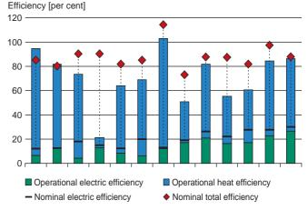
Nominal and operational efficiencies for 13 grate fired biomass CHP systems. Operational figures are average values for 24 months, September 2003 to August 2005.
