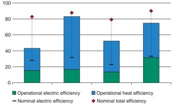
Nominal and operational efficiencies for 4 biomass gasification CHP systems. Operational figures are average values for 24 months, September 2003 to August 2005.
