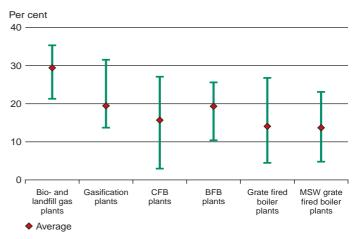
Comparison of min, max and average electric efficiency for the different technologies based on operational performance data for 24 months.
