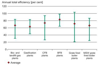
Comparison of the total of electric and heat efficiencies for the different technologies based on operational data for 24 months.
