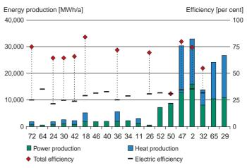
Operational efficiencies for 19 biogas and landfill gas CHP systems compared to the size of the plant shown as the annual production of electricity and heat. Operational figures are average values for 24 months, September 2003 to August 2005.
