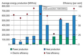
Operational efficiencies for 10 CFB biomass CHP systems compared to the size of the plant shown as the annual production of electricity and heat. Operational figures are average values for 24 months, September 2003 to August 2005.
