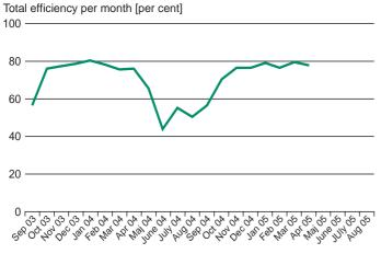
Total of heat and electric efficiencies for the dust-fired CHP plant. Figures are monthly data shown for 24 months, September 2003 to August 2005.
