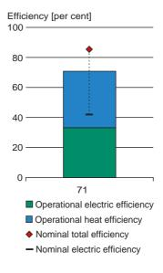
Nominal and operational efficiencies for the dustfired CHP plant. Operational figures are average values for 24 months, September 2003 to August 2005. Both electric and heat efficiencies are significantly lower in actual operational data compared to the plant nominal data.
