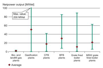
Comparison of the size, shown as min, max and average net electric capacity, for the different technologies.
