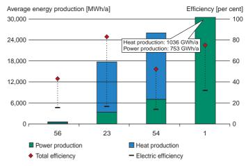
Operational efficiencies for 4 biomass gasifier CHP systems compared to the size of the plant shown as the annual production of electricity and heat. Operational figures are average values for 24 months, September 2003 to August 2005.
