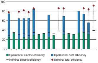
Nominal and operational efficiencies for 18 biogas and landfill CHP systems. Operational figures are average values for 24 months, September 2003 to August 2005.
