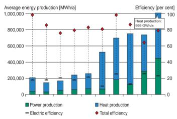
Operational efficiencies for 10 BFB biomass CHP systems compared to the size of the plant shown as the annual production of electricity and heat. Operational figures are average values for 24 months, September 2003 to August 2005. The electric efficiency is not impressive, less than 30% in most cases.
