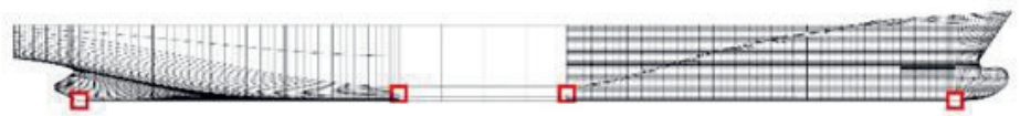
Figure 4. A detailed 3D panel grid is used to represent the full geometry of each vessel. Six points shown as red squares are placed strategically along the vessel hull to track minimum UKC requirements.
