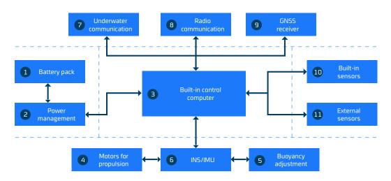
Figure 4: Reference architecture for an underwater drone. The drone consists of components numbered from 1 to 11.
