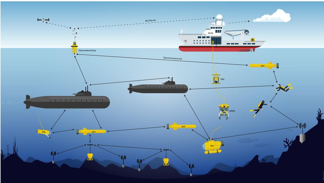
**Figure 3:** An overview of possible underwater drone technologies and the means of communication between them. For instance, from the cloud to sensors anchored in the ocean floor, in the case of nodes and sensor technologies with many communication lines.
