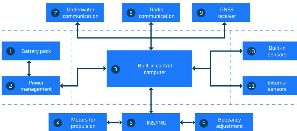
**Figure 4:** Reference architecture for an underwater drone. The drone consists of components numbered from 1 to 11.
