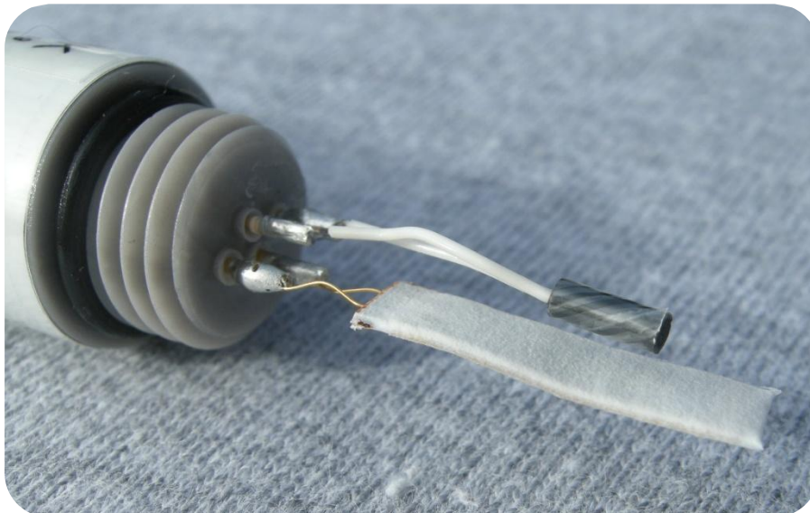
Figure 8: Humidity measurement probe without protection cap. Top: temperature sensor. Bottom: capacitive humidity sensor.
