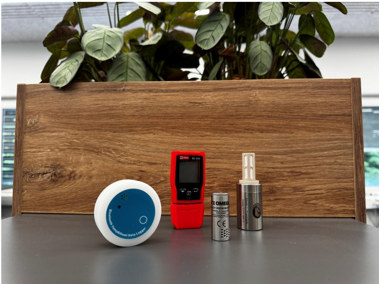
Figure 10: Data loggers for temperature and humidity measurements. From left: DBT-H90, RS-191A, OM-CP-MICRORHTEMP and TrackSense Pro.
