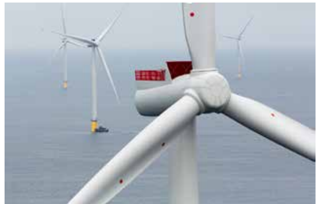
Figure 1: Increased rotor blade length benefits in a higher energy production for the wind turbine, but at the same time also increases the risk of leading edge erosion. The latter being a serious challenge for the wind energy industry.
