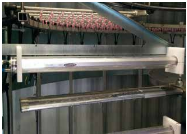
Figure 1: One of 3 blades in the RET tester parked between the two photo lights.
