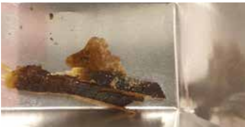
Figure 9 Wing material after treatment in supercritical reactor with a reactant ratio of 1:10 at 130 C. 3D decomposition has occurred.
