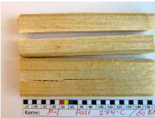
Figure 3 Example of decomposed polyester-based fiberglass after sub critical water solvolysis from LM
