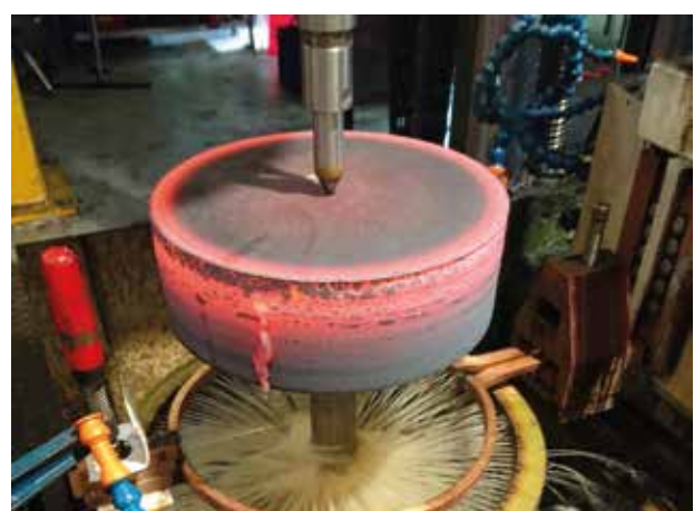
Figure 3: Induction heating of \varnothing 300 mm test sample.
