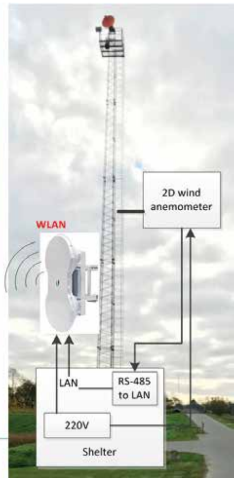
Figure 3b: Remotely placed 2D wind anemometer
