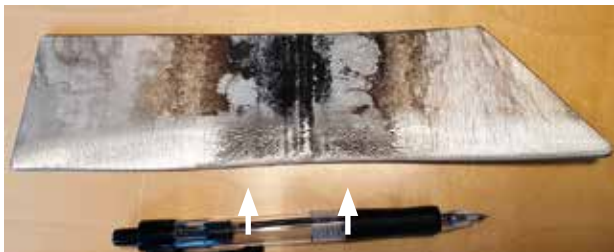
Figure 1: Sample from old vessel with pitting corrosion in the vicinity of a weld.
