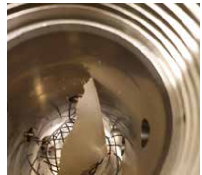
Figure 7 Polyester based wing material loaded in super critical CO2 reactor
