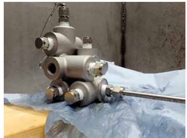
Picture 3: The valve housing after testing at approx. 1500 bar
