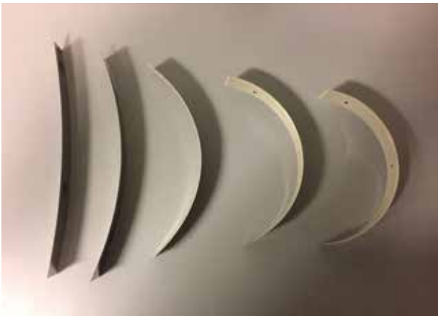
Figure 1: Bending increased with increase of dry film thickness
