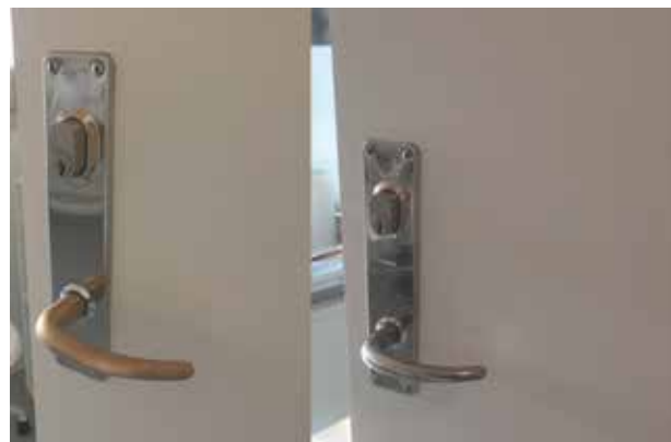
Coated and uncoated door handles during the field test in Kvistgaard, Denmark.
