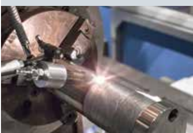
Fast Track 10: Surface treatment of cast iron
