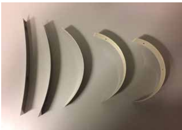
Figure 1: Bending increased with increase of dry film thickness
