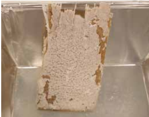
Figure 8 Wing material after treatment in supercritical reactor with a reactant ratio of 1:2 at 130 C. Surface reactions has occurred.
