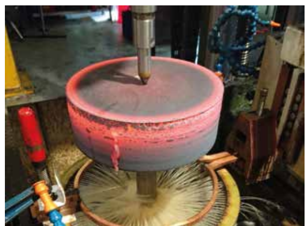
Figure 3: Induction heating of \varnothing 300 mm test sample.
