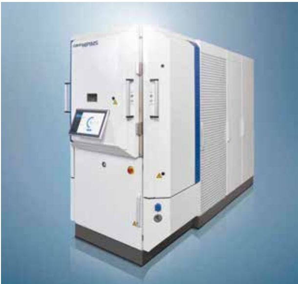
Figure 1: New HiPIMS coating equipment used for coating development and production.
