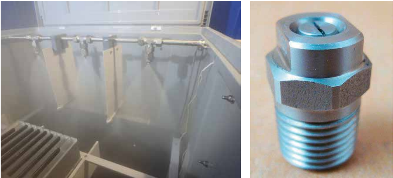
Figure 1 Left: Spray chamber, with 3 flat spray nozzles during a test. Right: Close up of a untreated flat spray nozzle
