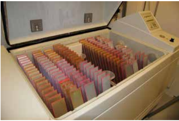
Figure 1: NSS test setup at DTU
