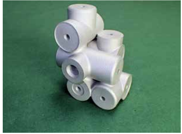
Picture 2: The 3D printed valve housing after glass blasting
