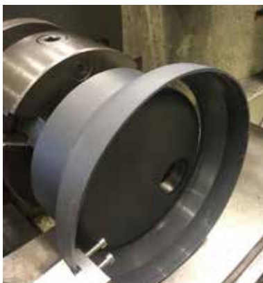
Figure 2: Accelerated wear test of the surface in a lathe.
