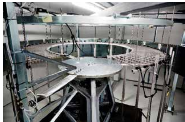
Figure 1: Rain erosion tester (RET) from R&D A/S
