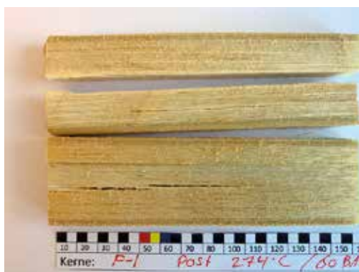
Figure 3 Example of decomposed polyester-based fiberglass after sub critical water solvolysis from LM
