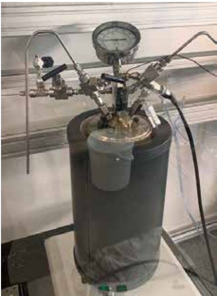
Figure 1 PARR reactor setup
