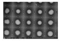
Integrated THz optics can drastically improve the performance of THz devices. The image shows microstructured substrate lenses for THz emitter arrays
