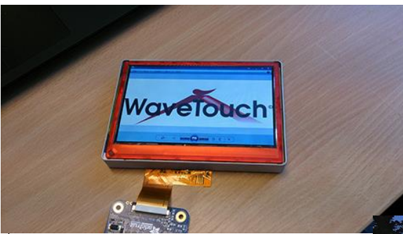
↑ Optical touch screen based on TIR in plastic or glass. It works embedded in water as well. ↓ WaveTouch Group Limited
