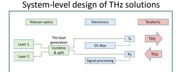
One of our other related focus areas is system-level design of more complex continuouswave THz systems using commercially available parts and devices to increase power and sensitivity.
