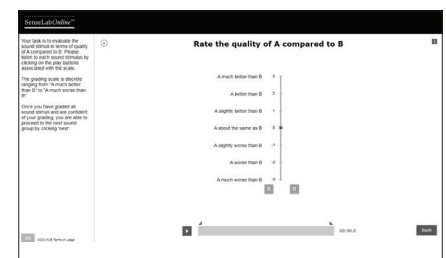
The SenseLabOnline implementation of the ITU-T P.800 CCR. A system (technology under test) is being rated on degradation against reference case.
