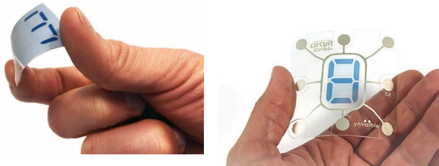
Figure 5: Examples of printed electrochromic displays
