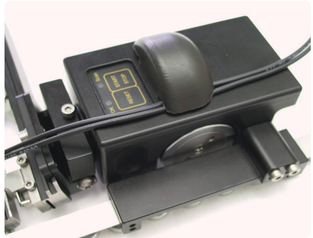
Hand support with integrated cable holder.
