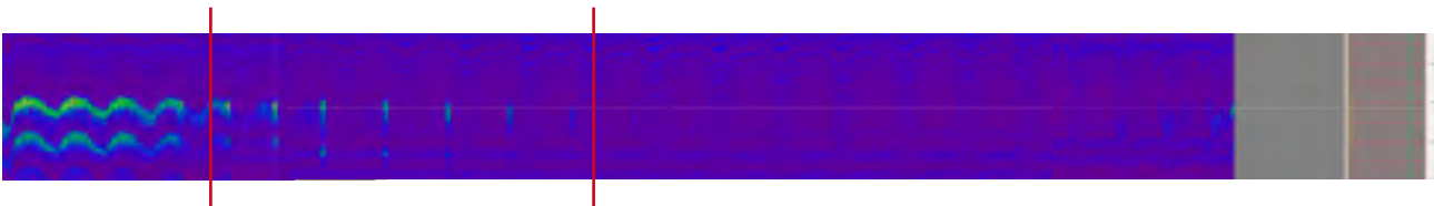
Figure 2 shows signals from a root defect in the welding (between the red lines)
