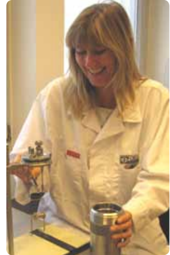
Preparing a sample of 1 g to determine calorific value
