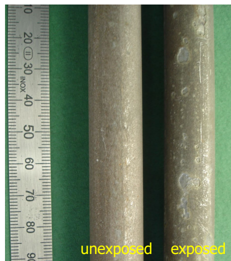
Figure 6: Cleaned surface of full-length coupon showing only minor corrosion after 1 year of exposure.
