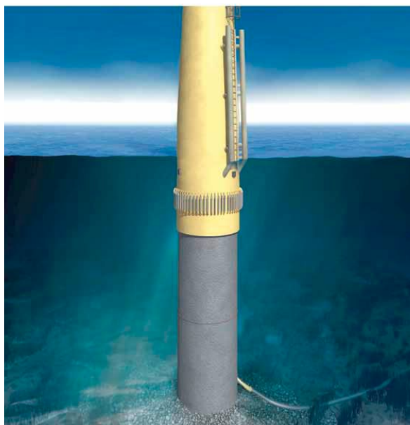
Figure 1: A principle sketch of a monopile-based design. The grey part is the monopile, the yellow part is the transition piece.
