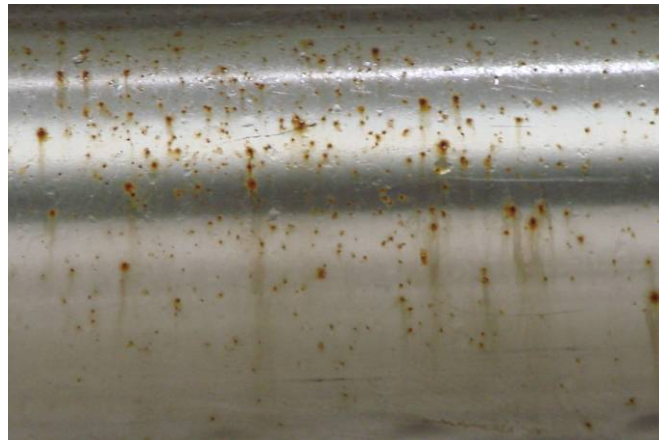
FIGURE 7 – Iron contamination from airborne grinding dust on the exterior of tubing.
