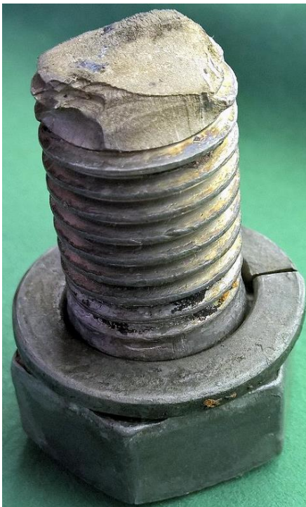
Figure 5: Fractured M20 bolt exposed to 2 years of subsea service.
