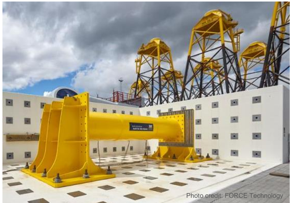
Figure 4: Full scale mechanical testing of critical parts of the new jacket design.
