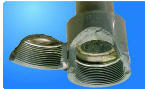
Environmental stress cracking in a PVC coupling
